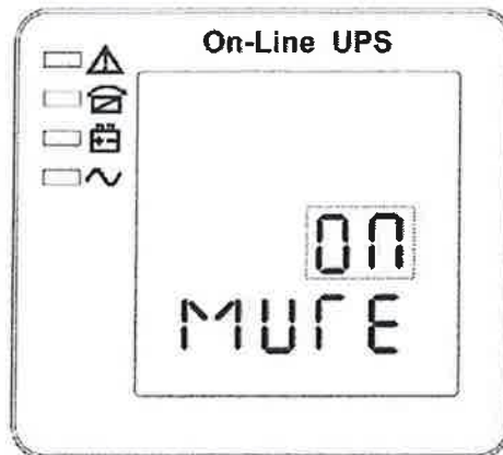
Buzzer Settings (note: red dashed box is the scintillation part)
