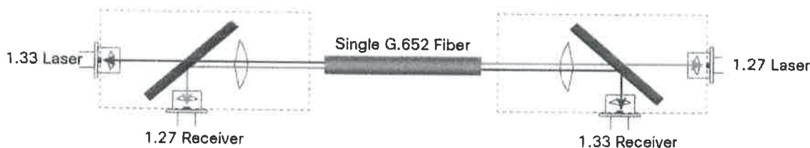
Figure 2. Bidirectional transmission of a single strand of SMF
