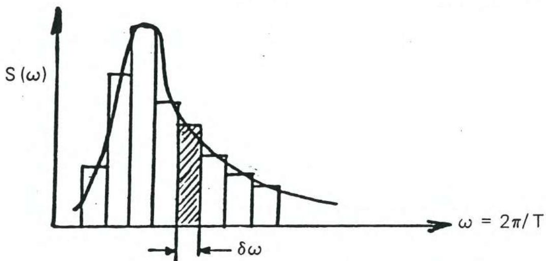
Each incremental area represents the wave energy in that incremental band of circular frequencies, i.e.  $dE = \rho g S(\omega_n) d\omega_n$ .
