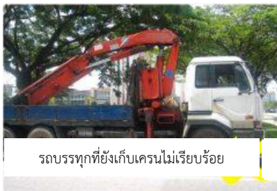
Lorry with crane partially retracted
